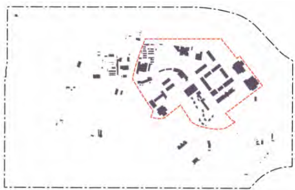
The Floor Area Ratio (F.A.R.) of the core, shown by the dotted red line, was 0.18 in 2000.
